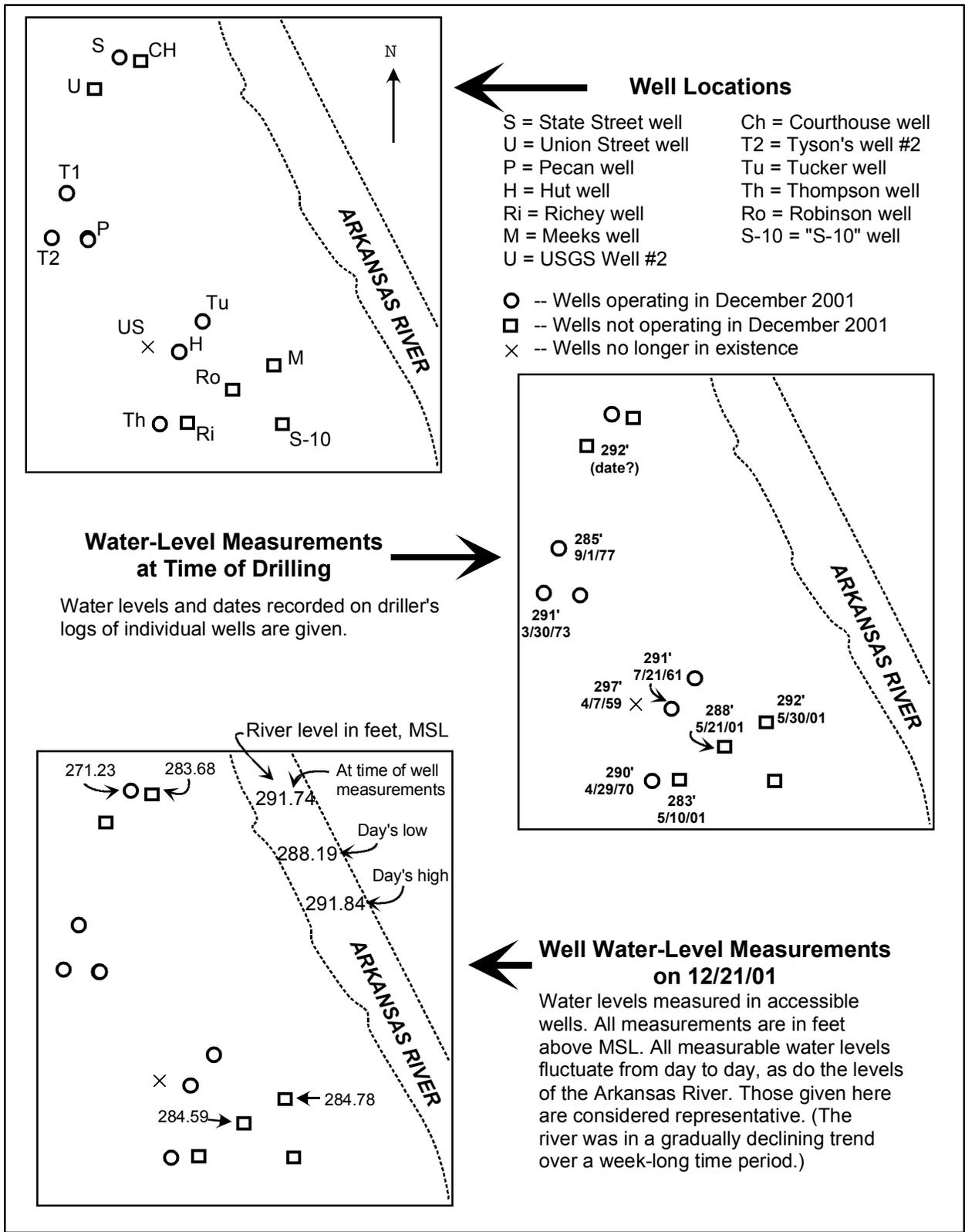
Figure 11. Maps for comparing model head distribution with water level measurements in wells and the Arkansas River.
