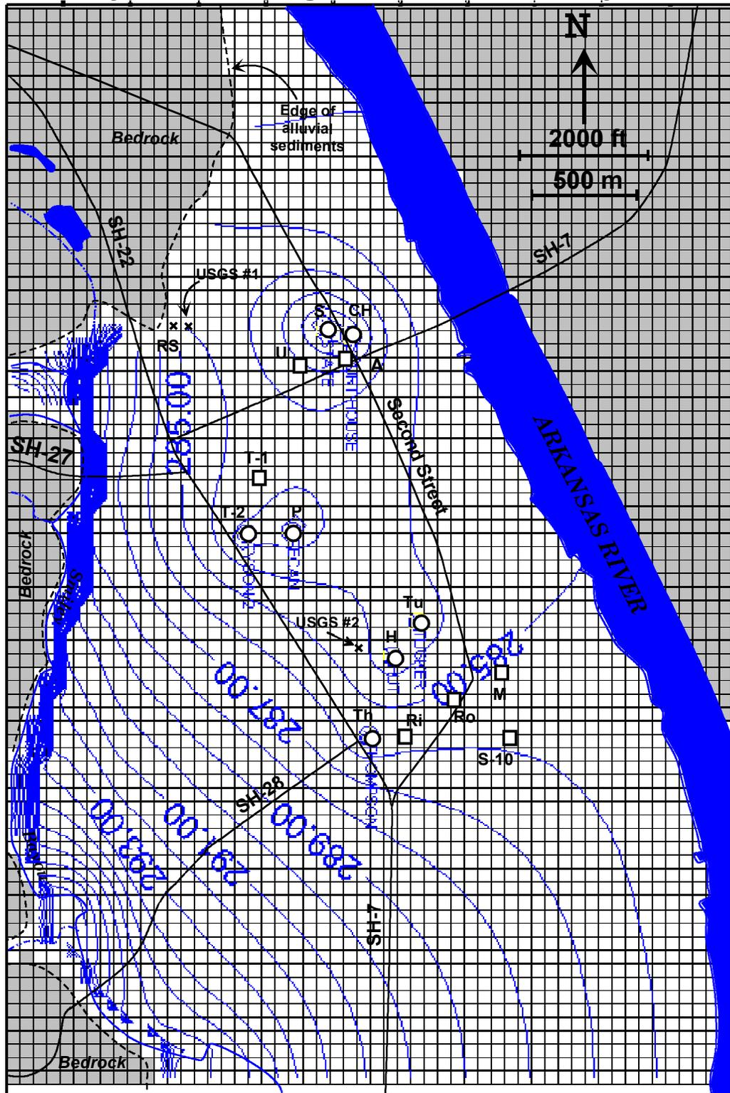
**Figure 10.** Potentiometric surface map generated by the steady-state groundwater model employing  $K = 400$  ft/d (122 m/d) in Layer 2. Contours are in feet above MSL; contour interval is 1 ft. Head in the Arkansas River is 285 ft (87 m). This map shows the condition when the wells are operating.
