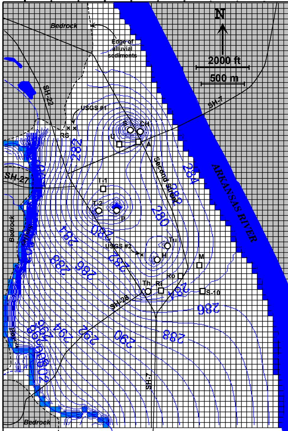
**Figure 8.** Potentiometric surface map generated by the steady-state groundwater model employing  $K = 175$  ft/d (53 m/d) in Layer 2. Contours are in feet above MSL; contour interval is 1 ft. Head in the Arkansas River is 285 ft (87 m). This map shows the condition when the wells are operating.
