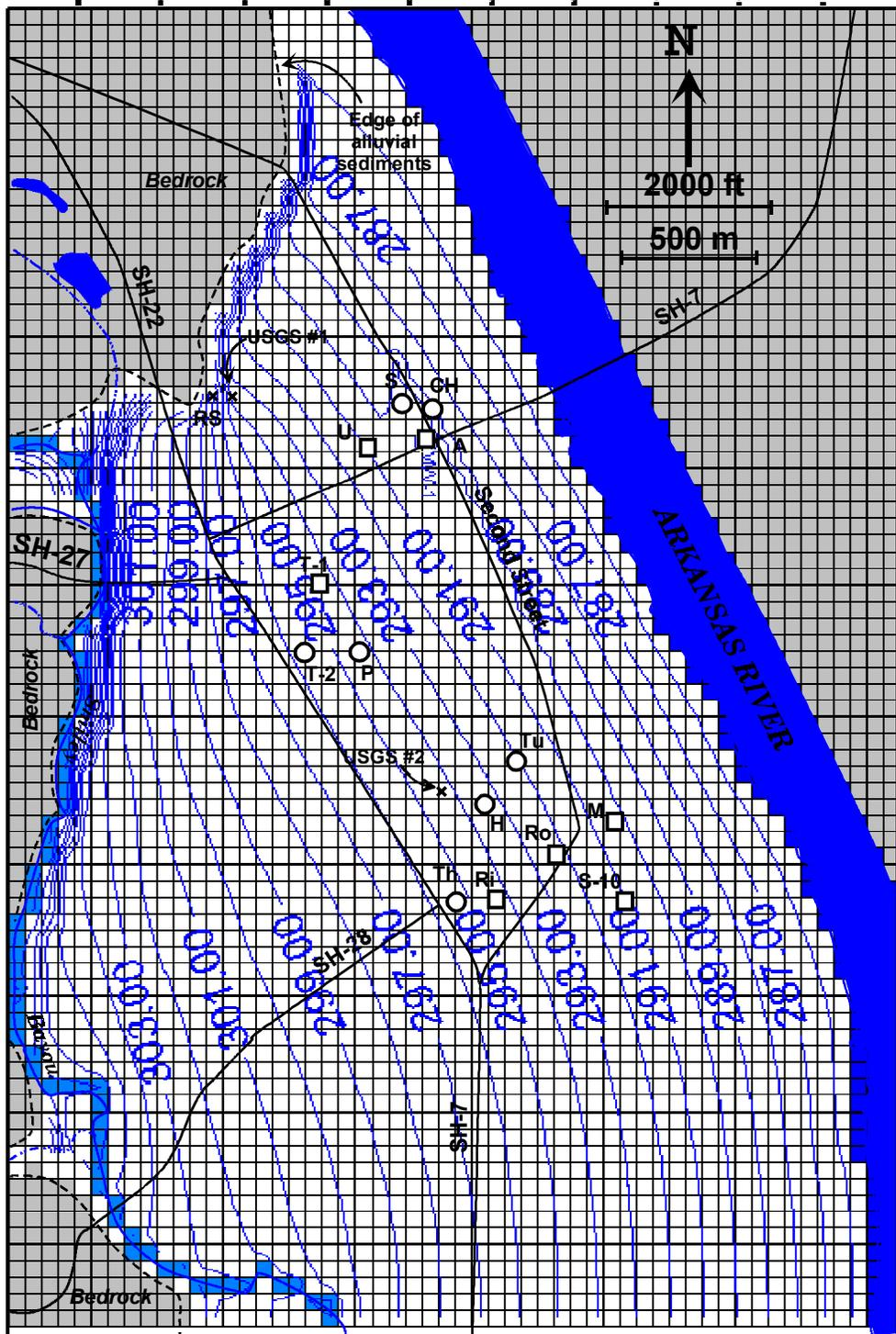
**Figure 7.** Potentiometric surface map generated by the steady-state groundwater model employing  $K = 175$  ft/d (53 m/d) in Layer 2. Contours are in feet above MSL; contour interval is 1 ft. Head in the Arkansas River is 285 ft (87 m). This map shows the natural condition, no extraction wells.
