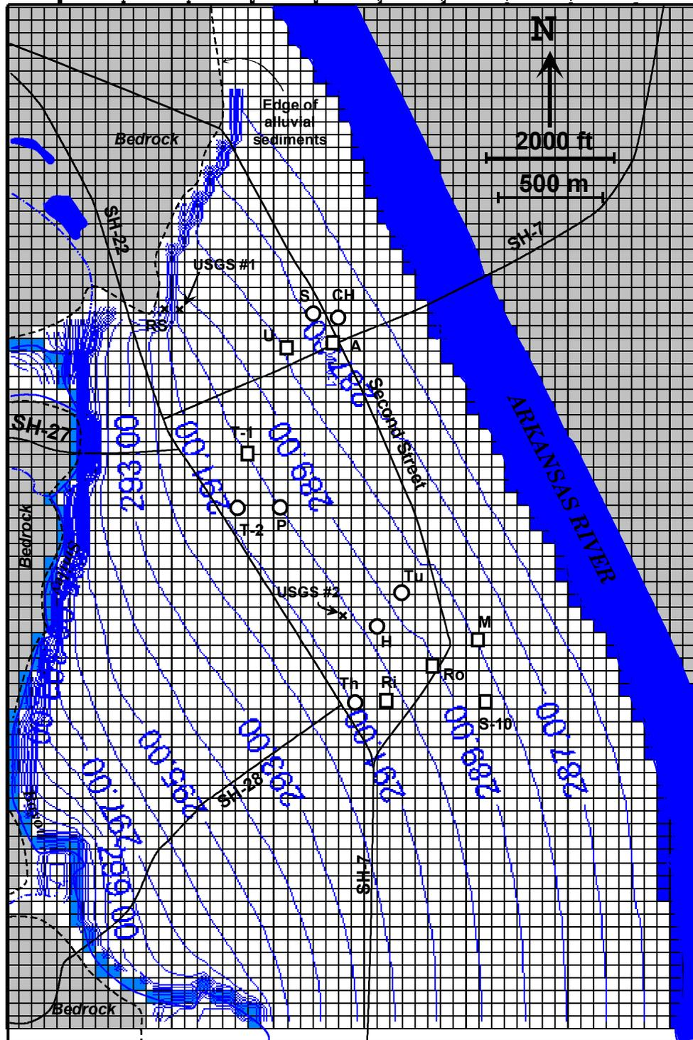
**Figure 9.** Potentiometric surface map generated by the steady-state groundwater model employing  $K = 400$  ft/d (122 m/d) in Layer 2. Contours are in feet above MSL; contour interval is 1 ft. Head in the Arkansas River is 285 ft (87 m). This map shows the natural condition, no extraction wells.
